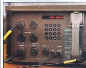
Channel status is displayed on the Deltamux front panel
